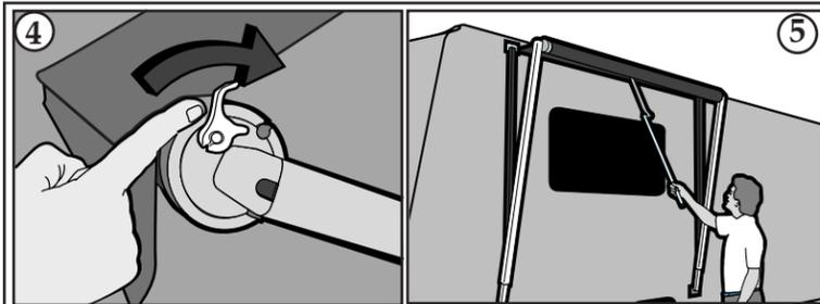
Grasp the pull strap, pull toward you, and flip the locking lever up to the ROLL UP position.
