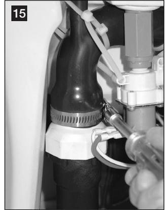
15. Position toilet over floor brackets and tilt toilet up from back. Push discharge assembly fitting and hose up into discharge loop outlet, and tighten band clamp (fig. 17).
