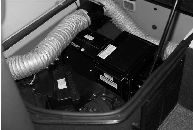
Figure 5: Example of ducting from plenum (Option 1: Two 4" flex ducts)
