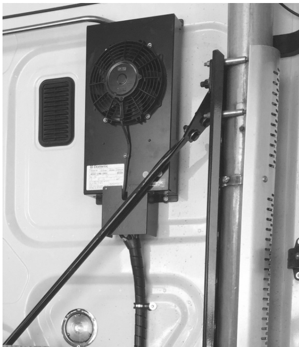
Figure 8: Condenser on Back of Truck
