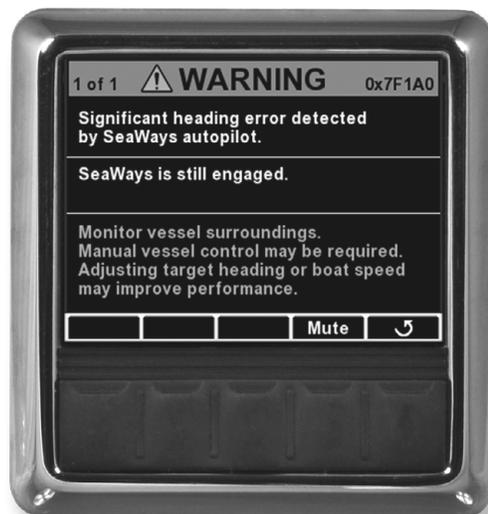
Figure 3-11. Heading Error 7F1A0.
