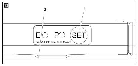
You can use the setting button (1) to set the cooling temperature to one of three values: 4 °C, 7 °C and 12 °C.
