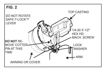
**2.** Carefully lay the fabric roller tube assembly on "V" troughs or other well protected surface to prevent fabric damage. Secure arm assemblies to the respective top castings using  $1/4-20 \times 1/2$ " hex. hd. machine screws and 1/4" lock washers. (FIG. 2)
