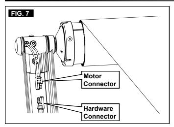
Connect 16 Gauge (minimum) wire leads (user supplied) to motor connector, and tape in place (with electrical tape).
