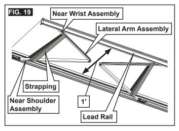
2. Tie all lateral arm assemblies securely (with fabric strapping or light rope) near shoulder and wrist. See (FIG. 19).
