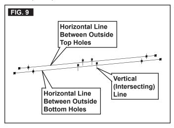
3. Verify horizontal lines are level. Then mark vertical lines from all remaining holes to intersect marked horizontal lines. See (FIG. 9).
