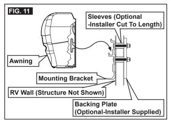
5. AWARNING IMPACTOR CRUSHHAZARD. Do NOT extend awning until it is securely [mounted / hooked] onto mounting bracket(s). Take special care when extending. Otherwise, awning could dislodge and fall. Failure to obey this warning could result in death or serious injury.
