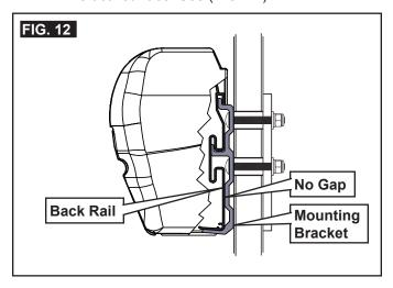
6. AWARNING IMPACT OR CRUSH HAZARD. Do **NOT** operate or leave awning unattended until it is securely fastened to mounting bracket(s). Otherwise, awning could dislodge and fall. Failure to obey this warning could result in death or serious injury.
