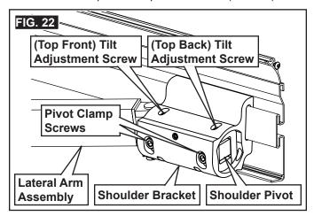
2. Support weight of lead rail and lateral arm assemblies securely.
