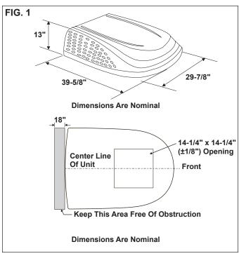
o. The roof must be designed to support 130 pounds when the RV is in motion. Normally a 200 lb. static load design will meet this requirement.
