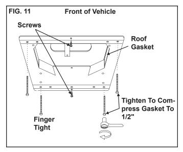
Evenly tighten the four mounting bolts to a torque of 40 to 50 inch pounds. This will compress the roof gasket approximately 1/2". The bolts are self locking so further tightening is not necessary. See FIG. 11.
