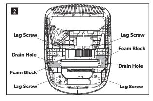
➤ Identify mounting hardware and drainage system components.
