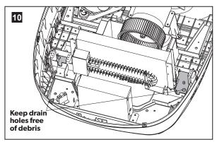
➤ Inspect the condensation drain area to ensure it is free of obstructions or debris that could clog the drain holes.
