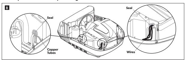
➤ Check seals around plumbing, tubes, and wires.
