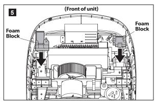
Ensure the foam cover blocks are installed over the drain holes. Use foam block kit no. 3316781.000 if foam cover blocks are not installed.
