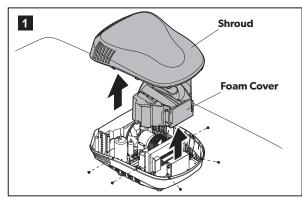
➤ Remove the foam cover and shroud from the unit.
