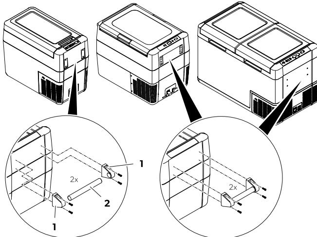
3. Fasten the handle with the enclosed screws in 2 of the waist shaped holes.
