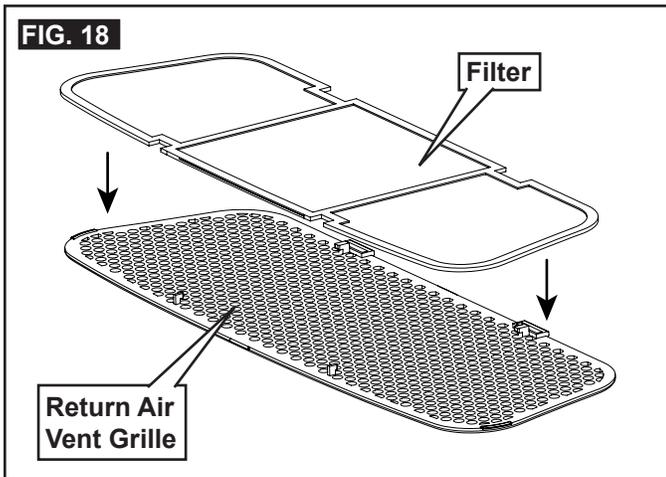
6. Install return air vent grille into the ADB. Slide return air vent grille tab into slot in ADB and rotate up and snap in place. See (FIG. 18).
