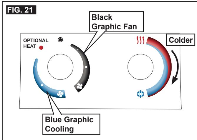
2. The thermostat controls the compressor On/ OFF operation within a temperature range of approximately 65° F and 90° F measured at the ADB inlet.
