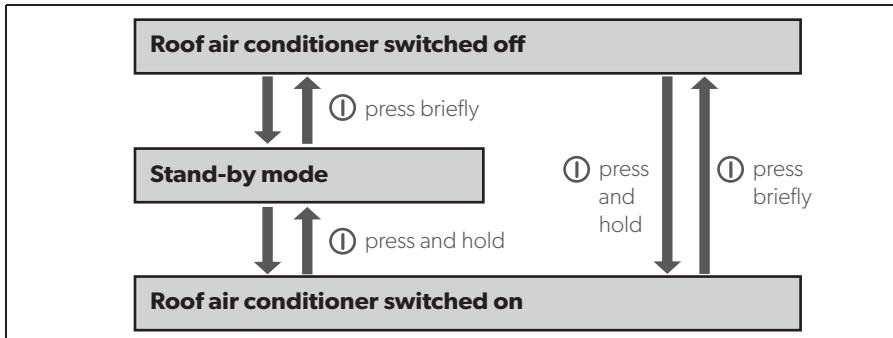
Example: The roof air conditioner is in stand-by mode. You want to switch it off.
