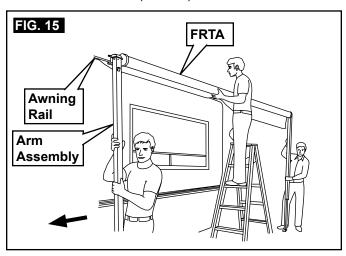
3. While one person guides awning fabric into awning rail, carefully move (carry) awning assembly to predetermined location. See (FIG. 15).
