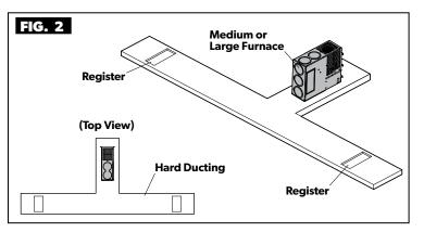
• Vertical Furnace – Bottom exit into hard ducting
