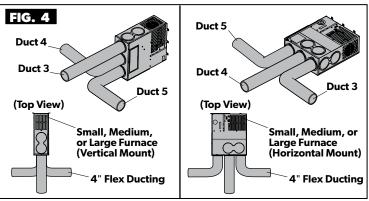
• Make sure to use at least the minimum number of 4" flex ducts required for your model size. See "Air Discharge Requirements" on page 11 and page 12.
