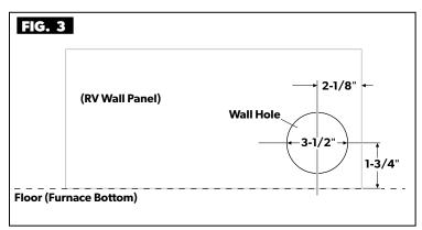
• There is **NO** door cutout on the outside of the RV for the small vent installation. The cutout is a hole in the side of the RV used to vent the Furnace outside of the RV.
