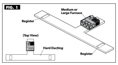
• Horizontal Furnace – Bottom exit into hard ducting
