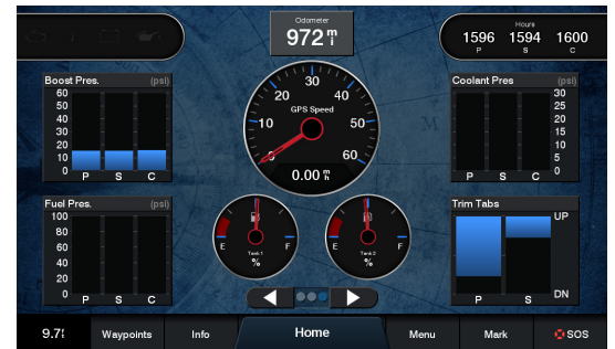
Trim tab position can be displayed on capable MFD's when adaptive dial controller is connected to public NMEA network
