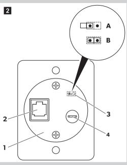
The remote control MCR9 is suitable to switch on/off the following inverters via the "Remote Port II" (also see the operating manual for the inverter):
