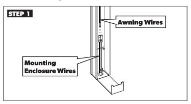
• Connect the black wire to the black wire and red wire to the red wire by stripping and crimping the wire splices.
