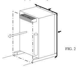
A wood strip must be in place across the upper opening of the enclosure. The top frame of the refrigerator will be anchored to the wood strip with screws.
