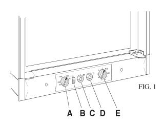
The refrigerator can be run on 230-240 V, 12 V or ULP gas. Changing between these modes of operation is carried out by means of the control buttons positioned as shown in Fig. 1.
