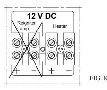
The connection is made to the positive (+) and negative (-) terminals of the terminal block. Correct polarity must be observed when connecting to the 12 volt DC supply. Do not use the chassis or the vehicle frame as one of the conductors.
