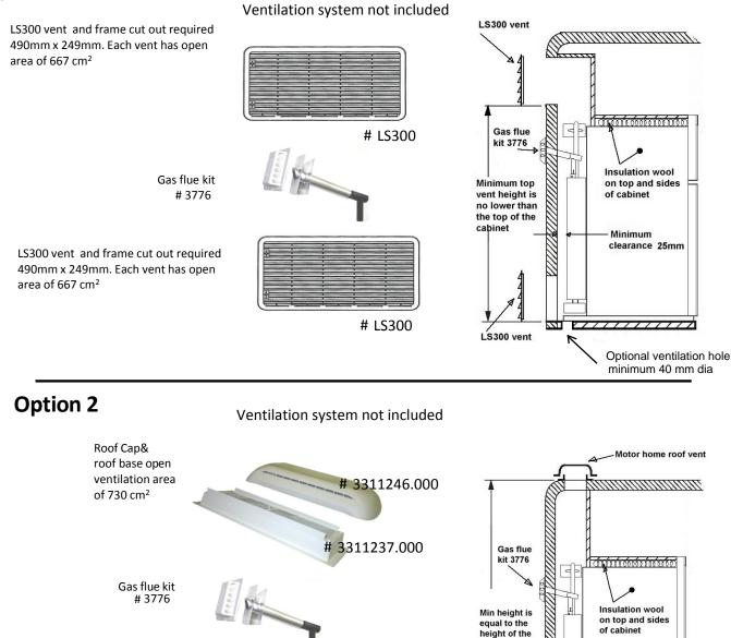
LS300 vent and frame cut out required 490mm x 249mm. Each vent has open area of  $667\ \mbox{cm}^2$
