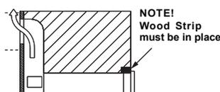
Push the refrigerator into the recess until the sealing strip on the flange seals against the front of the recess, so that the cooling unit is completely sealed off against the interior of the caravan.
