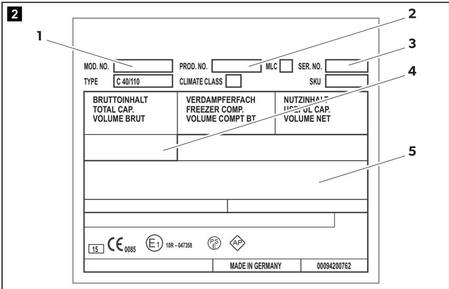
Inside the refrigerator you will find the type plate of the refrigerator. You can read the model name, product number and serial number there. You will require this information whenever you contact customer service or when ordering spare parts:
