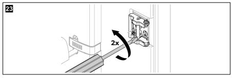
▶ Undo the two screws on the door lock and remove the door lock (fig. 23).
