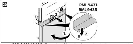
RML9431/9435: Open the refrigerator door and undo the screws underneath the control panel (fig. 20).
