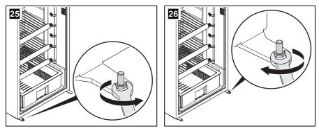
▶ Undo the hinge pin (fig. 25) and position it on the other side (fig. 26).
