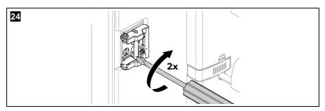
Place the door lock on the other side again and tighten it with the two screws (fig. 24).
