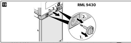
**RML9430**: Unscrew the dials carefully and loosen the screws (fig. 19).
