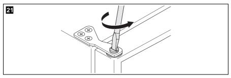
▶ Undo the hinge screw on the top door hinge and keep it in a safe place (fig. 21).
