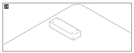
Make sure that the ventilation grille in the outer wall of the caravan or mobile home (fig. 16 1, page 7) and the roof vent (fig. 29) of the refrigerator are free of any dust and dirt, so that heat generated during operation can be released and the refrigerator is not damaged.
