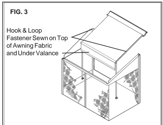
4. Fasten front of screen room to front by joining hook & loop fasteners together under valance. Pull side panels over rafters and join to fabric on top of awning on both sides.
