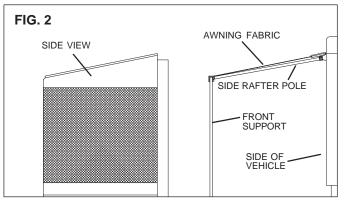
After awning is set up, remove screen room from storage bag and line up in position with awning as shown in FIG.
