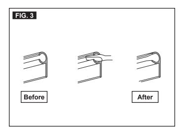
2. Unfurl fabric one revolution before installing awning fabric (with awning roller cover, if equipped) into awning rail. See FIG. 3.
