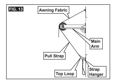
4. Using the strap hanger as a template, mark the strap hanger's position and hole locations.
