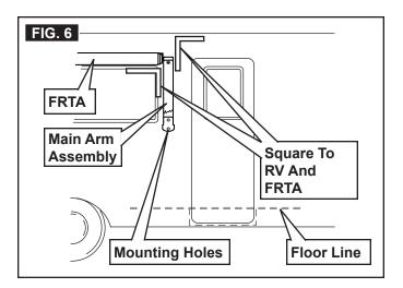
3. Use foot brackets to mark bottom mounting hole locations. See FIG. 6 and 7.
