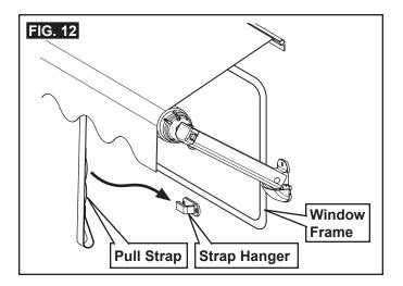
Locate strap hanger(s) so that the top loop of pull strap is engaged on strap hanger. This will allow for minor height adjustment of awning. See FIG. 13.
