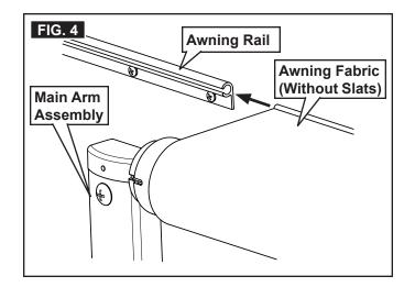
3. After awning fabric has been threaded into awning rail, check to make sure its position allows for solid mounting of the foot bracket, and that main arm assemblies are in desired location (not restricting use of doors, windows, etc.). See FIG. 5.
