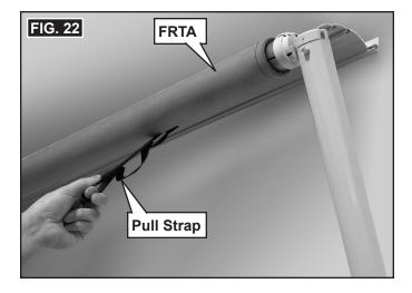
2. Hook pull strap's bottom loop onto strap hanger, then carefully and slowly allow awning to roll up until pull strap is taut. See FIG. 23.
