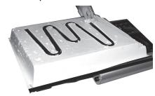
5. Apply thermal mastic to the coils.
