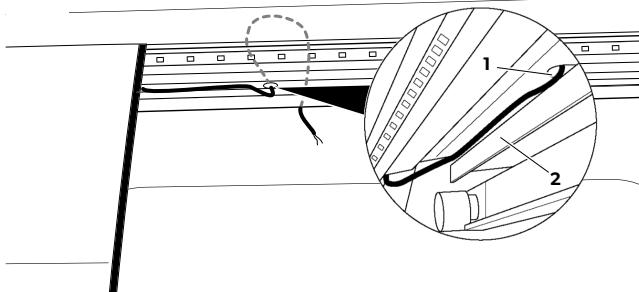
9. Place the connecting cable in the gap above the upper guide rail ( Fig. 7 on page 8, 2).
