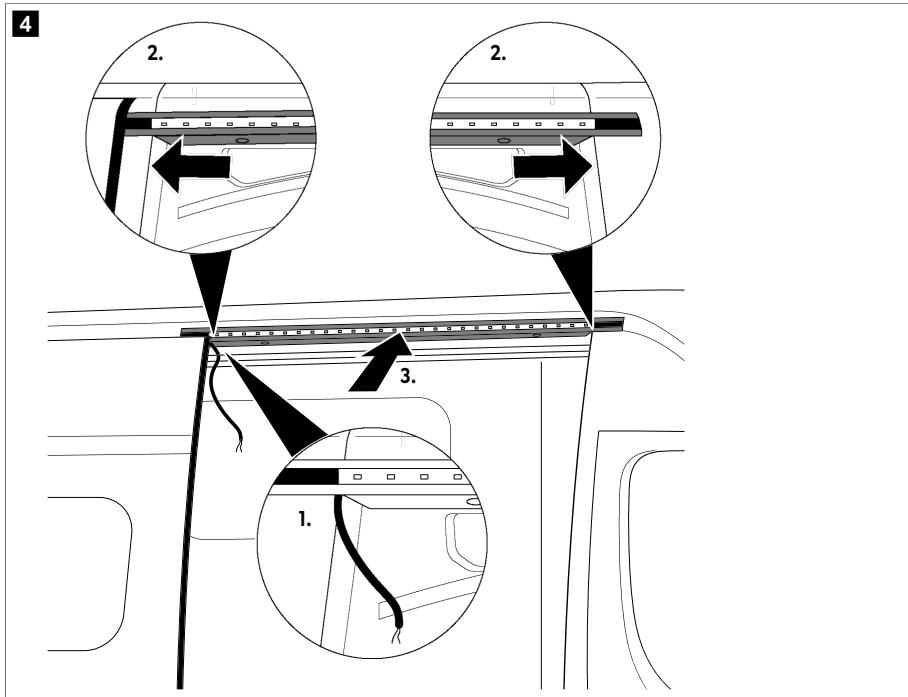
4. Align the rain gutter in the middle of the door opening using the sloping surfaces on both ends of the rain gutter ( Fig. 4 on page 6, 2).
