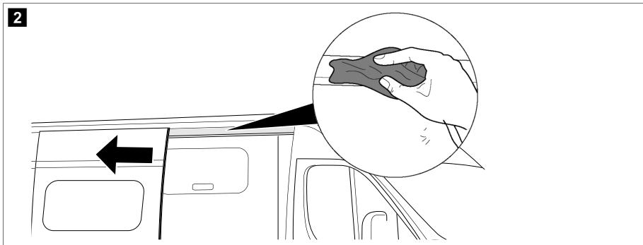
2. Remove the protective film from the adhesive strip.
