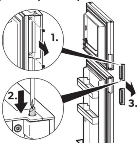
16. Remove the two screws (fig. 56 1.) from the latch assemblies on the freezer door and on the refrigerator door.
