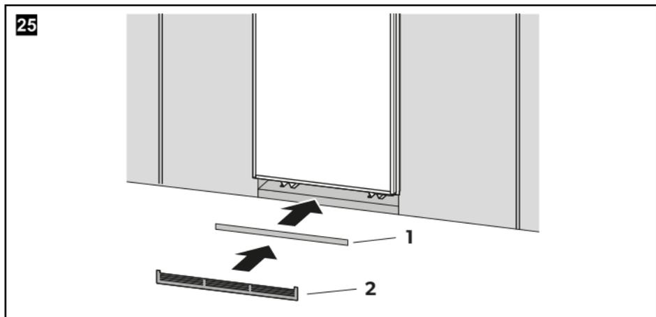
1. Apply a sealing strip (fig. **25 1**) along the bottom edge of the bottom grille (fig. **25 2**).
