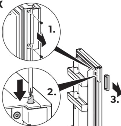
15. Remove the two screws (fig. **48 1.**) from the latch assembly.
