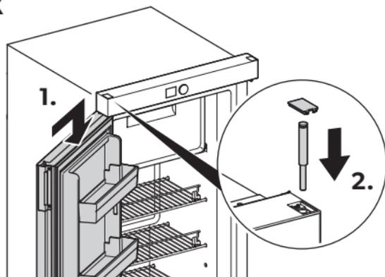
21. Insert the refrigerator door onto the bottom hinge pin at the new position on the opposite side of the door frame (fig. **49 1.**).
