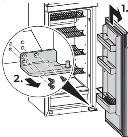
7. Remove the refrigerator door by lifting the refrigerator door over the bottom hinge pin (fig. 53 1.).
