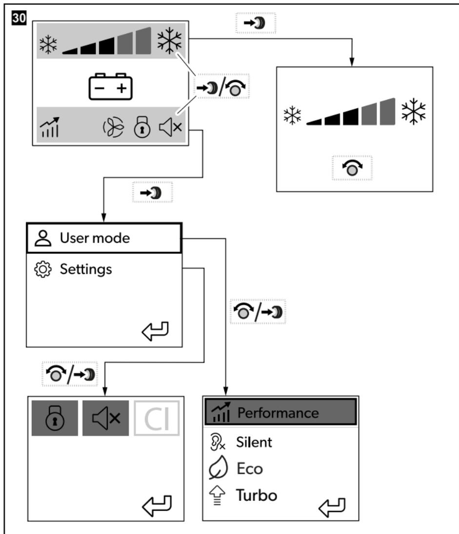
1. Rotate the control knob to select a submenu.
