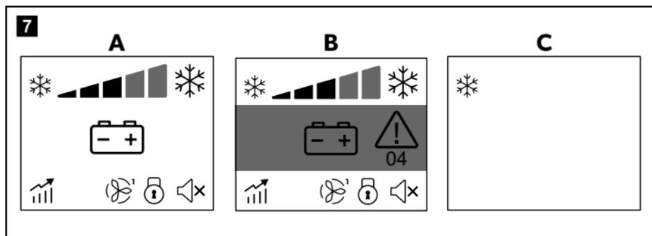
After 10 seconds without operating the control knob, the backlight dims and the display returns to the main menu (A). If activated, the child lock is active (see chapter "Setting the child lock (RUC 5208X, RUC 6408X, RUC 8408X only)" on page 39).
