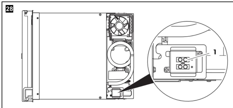
3. Protect the positive cable of the vehicle battery with a fuse:
