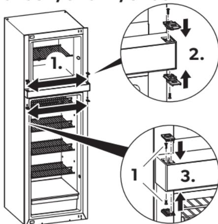
15. Attach the locking latches and the bushings to the opposite side of the door frame from their respective starting position (fig. 55).
