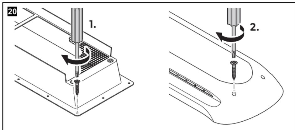
2. Insert the mounting frame into the prepared opening in the outer roof (see chapter "Installing the refrigerator" on page 20) and screw the mounting frame to the mounting holes (fig. **20 1**).
