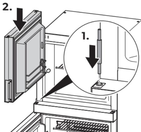
26. Insert the middle hinge pin and push it into the top of the refrigerator door (fig. 58 1.).
