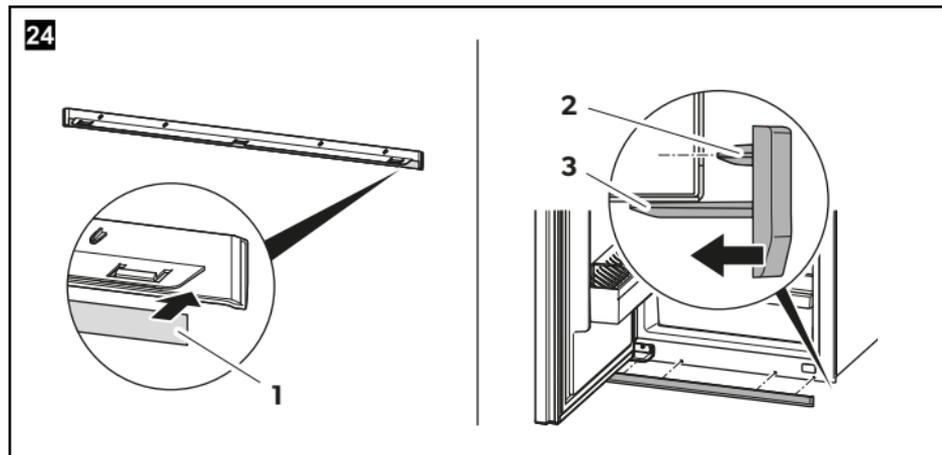
1. Apply a sealing strip (fig. **24 1**) to the lower surface of the bottom trim piece.
