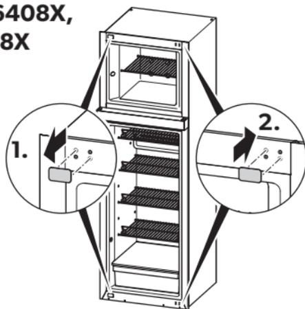
22. Remove the covers from the screw holes at the top and bottom hinge points using a small screwdriver (fig. 57 1.).
