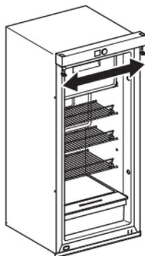
14. Attach the locking latch and bushing to the opposite side of the door frame from their respective starting position (fig. **47.**).
