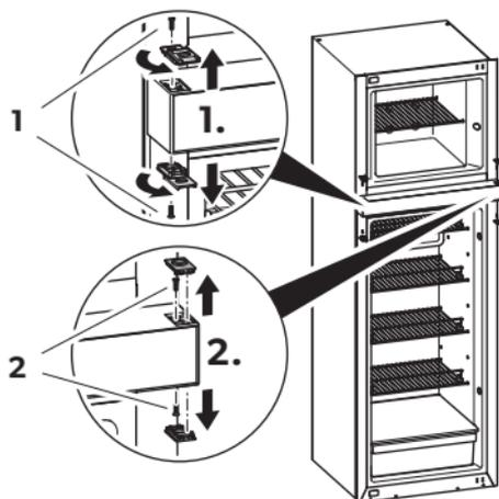
10. Turn the locking latches on the latch side by 180° to expose the screws.
