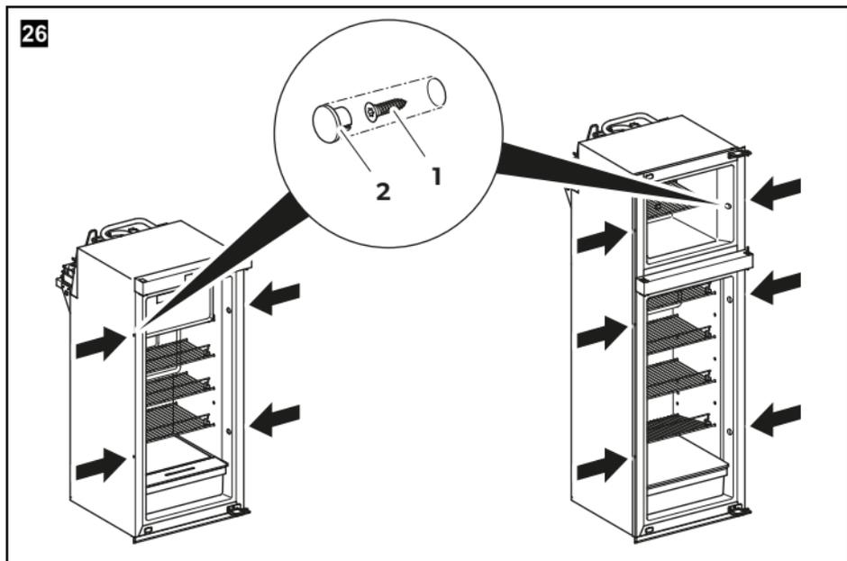
3. Insert the screws (fig. 26 1) through the plastic bushings on the sides of the refrigerator and screw the refrigerator into the recess.
