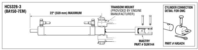
Figure 23. HC5326-3 (BA150-7EM), manual, non-power steering.
