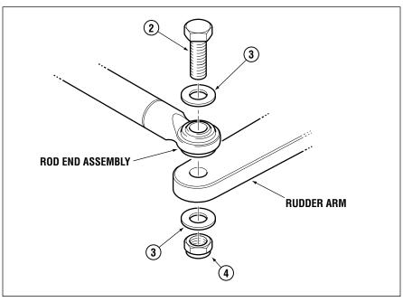
Figure 10. Attaching Rod End Assembly to Rudder Arm.
