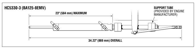
Figure 22. HC5330-3 (BA125-8EMV), manual, non-power steering.
