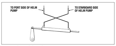
Figure 30. HC5332-2 Cylinders ONLY. Hoses are crossed when plumbing.
