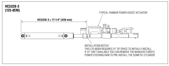
Figure 13. HC5328-3 (125-8EM) Yanmar, NOT for use with SeaStar PRO helm(s).
