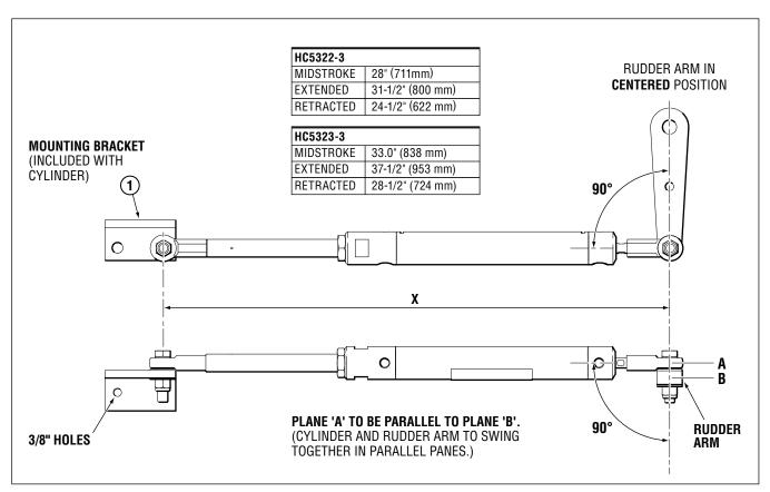
Figure 9. Correct Cylinder to Rudder Arm Mounting Orientation.
