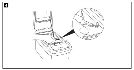
You can keep the lid of the cooler open by hooking the chain in the screws on the inside (fig. 4).
