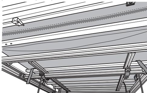
1. Use the screw driver and wrench provided in the tool bag to remove motor push rods from both sides.
