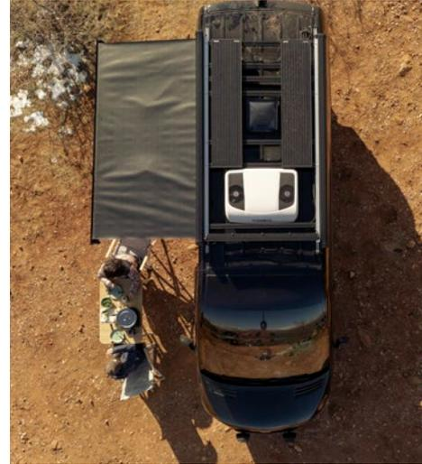
Dometic’s new ACC3100D rooftop ventilation system for RVs which not only sets a new standard in ventilation and indoor air quality, but also stands out for its remarkable effect on energy consumption.
